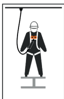
Fall Arrest Attachment Point Front Loops marked with ½ "A"
