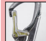
Gate does not close, even after cleaning.
