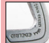
Significant material abrasion \geq 20\%
