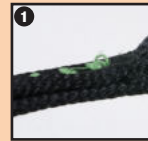
Individual loop has pulled
