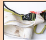
Energy absorber dirty/damp
