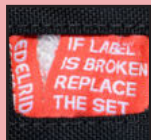
Safety label ripped
